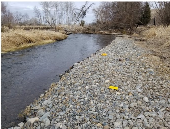
Figure 5 Sediment gradation of existing gravel bar in the reach. The gravel bar shown is located near the upstream end of the middle segment on the right bank of the main channel. Gravel bars typically reflect the bed material in active transport. The broader bed was observed to be generally coarser than gravel bars.
