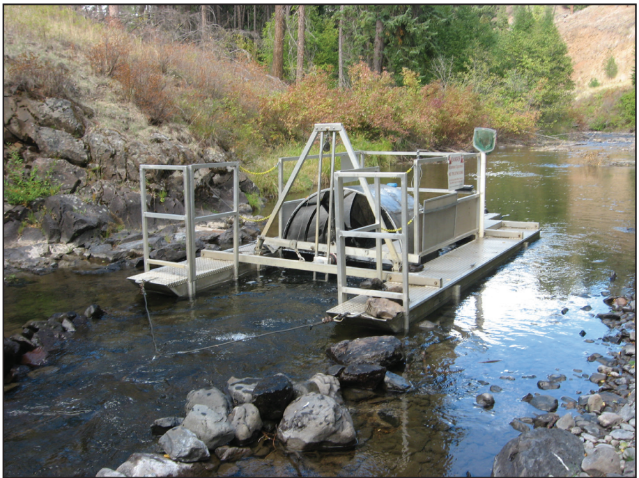
Above: ODFW staff use mobile receivers to track fish locations of Chinook fitted with radio tags. Below: The Upper Grande Ronde Rotary Screw Trap helps researchers estimate timing and abundance of outmigration for juvenile fish. (Photos: ODFW)
