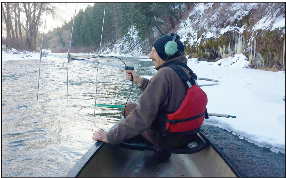
Above: ODFW staff use mobile receivers to track fish locations of Chinook fitted with radio tags. Below: The Upper Grande Ronde Rotary Screw Trap helps researchers estimate timing and abundance of outmigration for juvenile fish. (Photos: ODFW)
