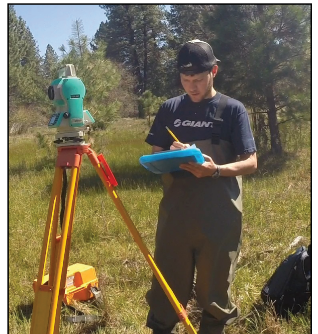
Above: An engineering student surveys the main channel of Catherine Creek. (Photo: GRMW)
