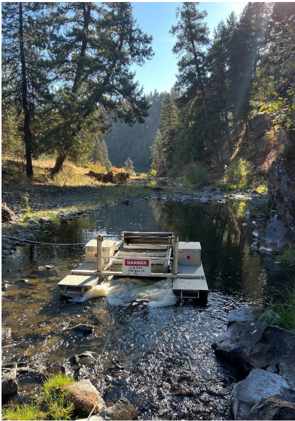
Figure 3: The Meadow Creek Incline Plane trap is a fish trap that is located at the lower end of the creek before it meets the Grande Ronde River. This trap is designed to catch fish as they move out of the watershed. The data from this trap will tell us how long a fish tagged upstream has spent in the watershed and we can tag any fish not already caught higher up. From these data we will be able to estimate the number of out-migrating salmonids and monitor their survival down through the Columbia River. Downstream of the trap is a PIT tag receiver array that adds another layer of detection for fish going out but also detects tagged fish coming back into the system. (Courtesy of Jacob Kennedy, CTUIR Grande Ronde Research, Monitoring and Evaluation)
