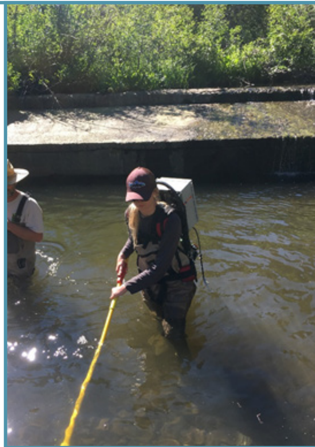
Interns conducting fish salvage on Beaver Creek using electrofishing equipment (courtesy of Confederated Tribes of the Umatilla Indian Reservation).
