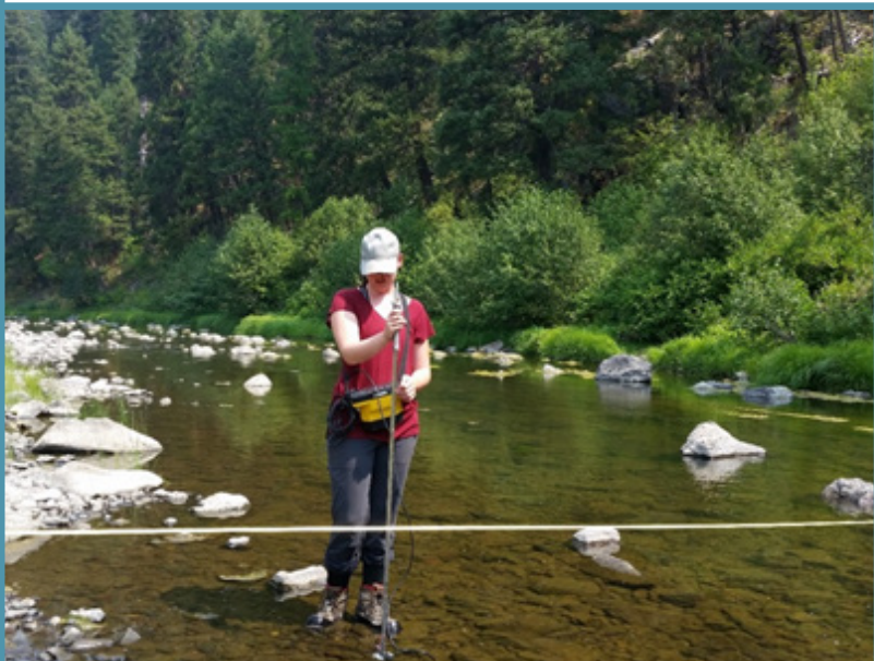
A BOR intern collects flow measurements on the Grande Ronde River (courtesy of BOR).
