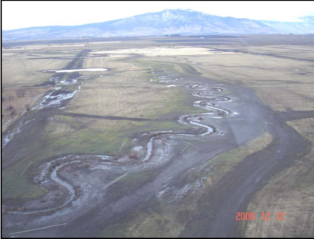
Upstream reach of End Creek (Rice) Restoration Channel, viewing east (downstream) towards South Fork Willow Creek confluence. Note reclaimed channelized reach in left corner of photo and floodplain ponds incorporated into reclamation plan
