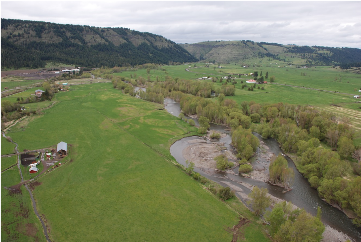
Figure 8. Aerial photo of Wallowa-Baker Project looking downstream, 2012. New channel carved on right bank and left bank channel now only activated at high flows.
