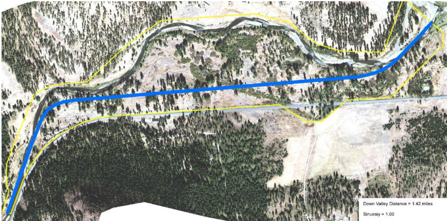
Figure 5-9 Theoretical Minimal Length, Single Thread Channel
