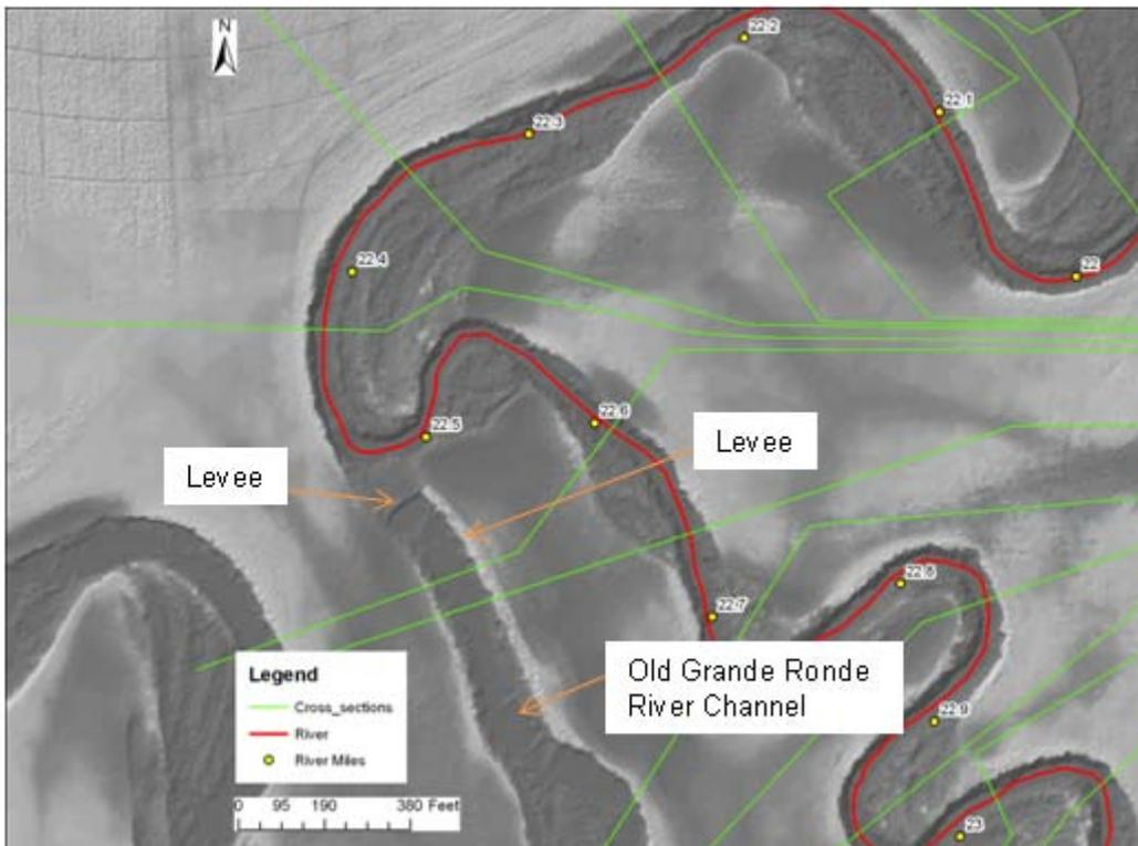
(higher velocities for greater discharges) upstream of Ladd Creek. The reach-averaged velocity increases from approximately 2.7 ft/sec for the 1.5-year flood to 3.3 ft/sec for the 100-year flood.
