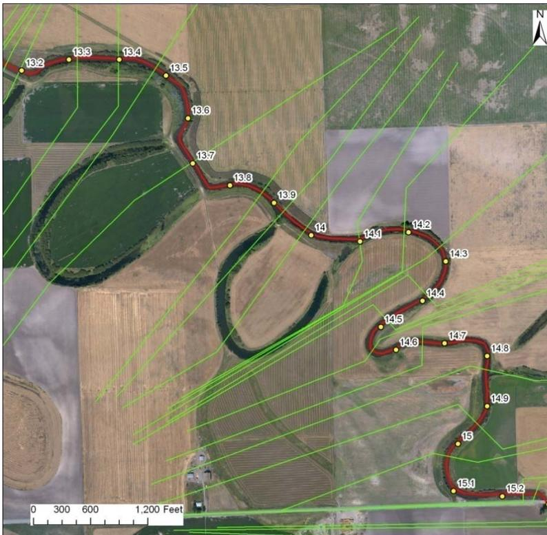
Figure 50. Oxbow at RM 14 that is inundated by the 1.5- year flood.
