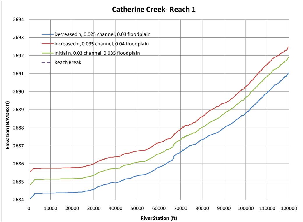
Figure 23. Sensitivity to Manning's n at a 1.5 year discharge for Reach 1 of Catherine Creek.
