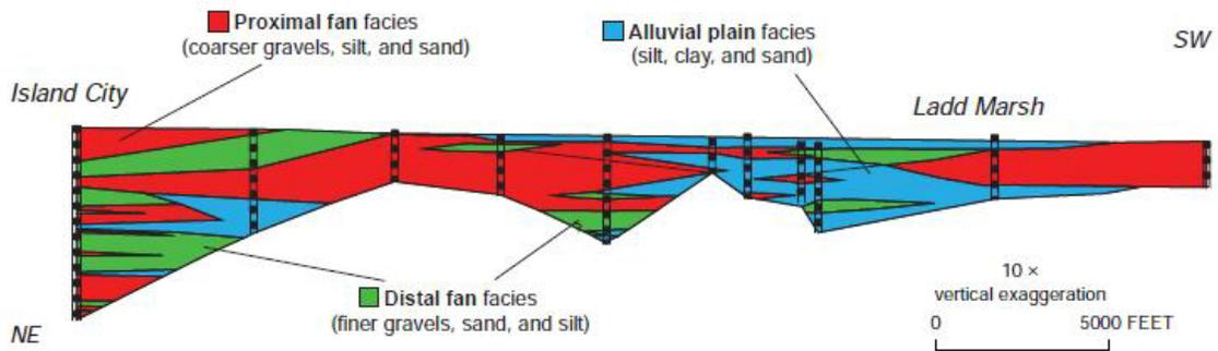
**Figure 1. Interpretive cross section in the Grande Ronde Valley (Ferns et al. 2010).**
