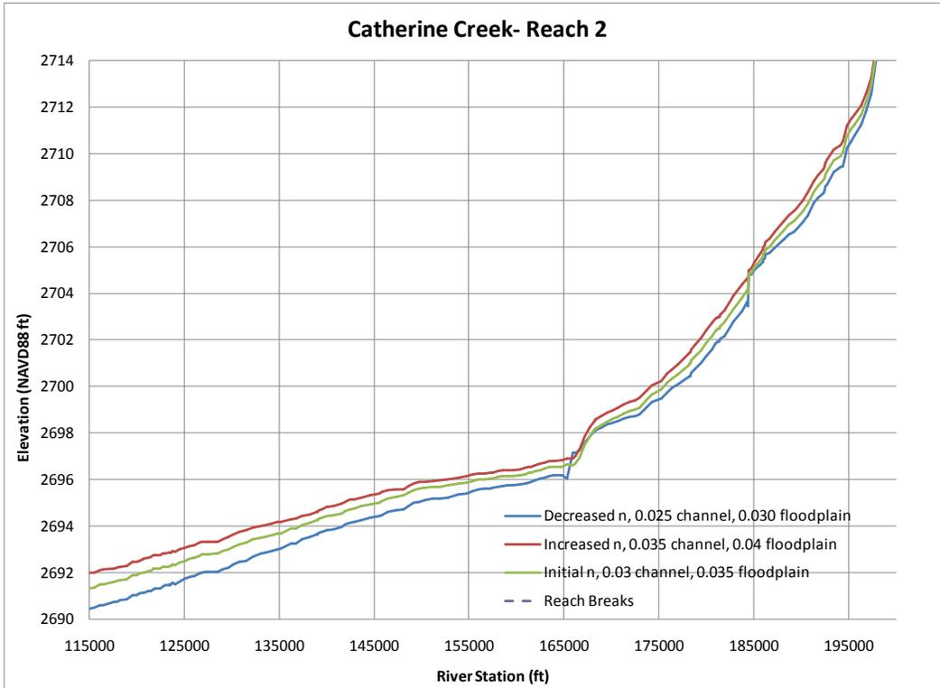
Figure 25. Sensitivity to Manning's n at a 1.5-year discharge for Reach 2 of Catherine Creek.
