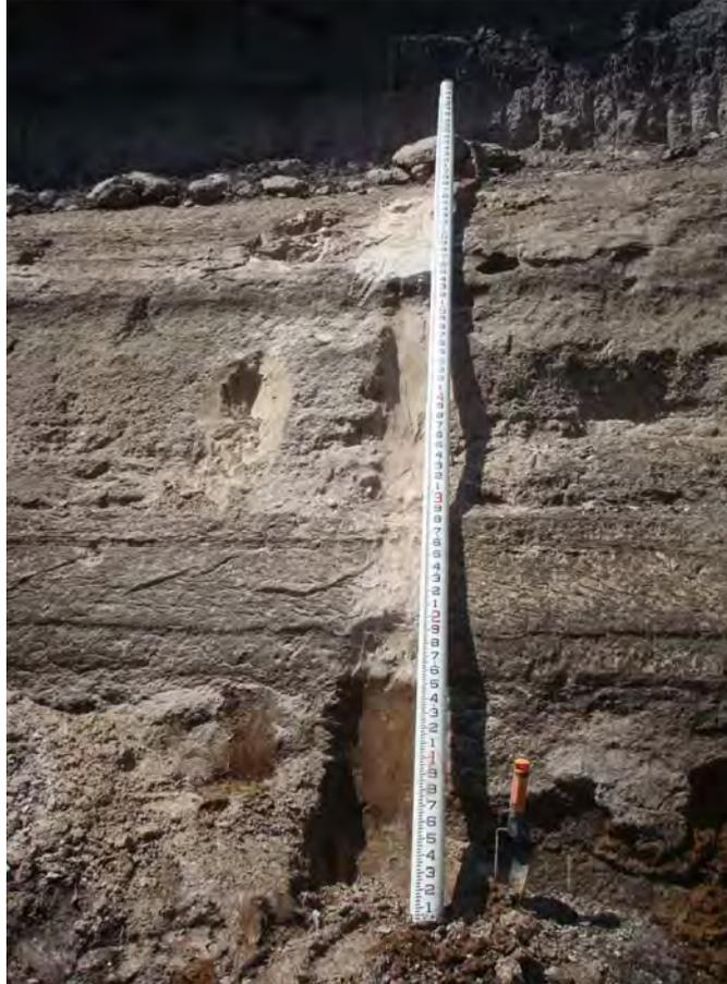
**Figure 17. Close up of stratified fine-grained fluviolacustrine sediments (Qal1) exposed on the bank of Catherine Creek at RM 22.70, material consists of brown silty sand (SM) overlain by firm to hard light colored sandy silt and diatomaceous silt. Catherine Creek TA-Grande Ronde River Basin-Tributary Habitat Program, Oregon – Bureau of Reclamation – July 30, 2010.**
