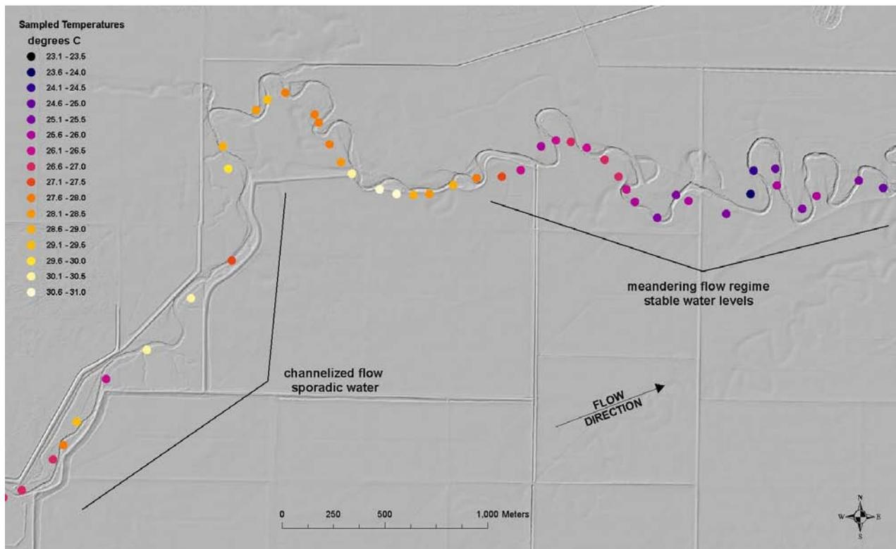
**Figure 9.** LiDAR bare earth hillshade that shows the transition between the confined, channelized river and the sinuous meandering channel near RM 29.1. Along this portion of Catherine Creek, water levels begin to rebound and a 6.4°C temperature decrease is seen in the lower 5 miles of reach 2 as the river returns to a more natural flow regime. The point color ramp is exaggerated for this image (Watershed Sciences 2010).
