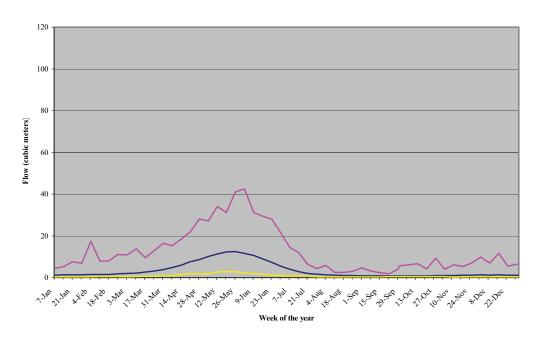
**Figure 4.** Hydrograph of Mean Flows in Catherine Creek near Union 1911-1996. The bottom line (yellow) represents minimum; the middle line (blue) mean; and the upper line (purple), maximum flows.
