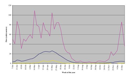
**Figure 3.** Hydrograph of Mean Flows in the Upper Grande Ronde River near Hilgard 1937-1955 and 1966-1981. The bottom line (yellow) represents minimum; the middle line (blue) mean; and the upper line (purple), maximum flows.
