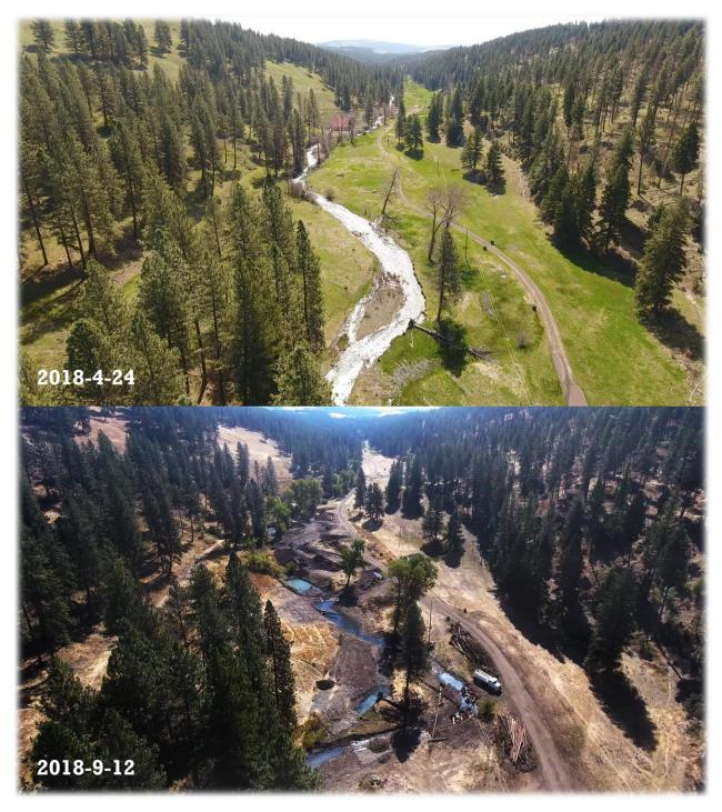
A tributary to the Upper Grande Ronde and an important steelhead stream, Rock Creek is on private land. Prior to restoration, Rock Creek exhibited high width to depth ratio and was incised throughout most of its length. CTUIR Habitat Program, working with the landowner, improved sinuosity and floodplain connection as well as narrowing the channel. This project was funded primarily by BPA and will be completed in 2019. Photos by Connar Stone (GRMW).
