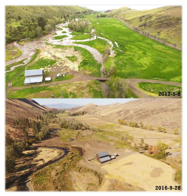
CC 44 Southern Cross. Sponsor: CTUIR. Funders: BPA, CTUIR. Completed: 2016. Photos by Connar Stone (GRMW), Catherine Creek Subbasin. Bottom photo shows recently constructed main and side channels during low flows. Upper photo demonstrates floodplain and side channel activation at higher flows.
