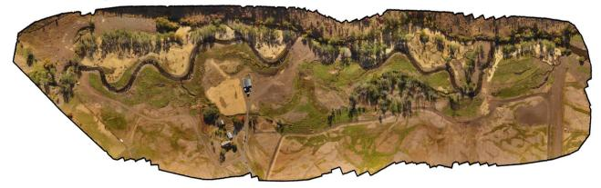
CC 44 Southern Cross. Sponsor: CTUIR. Funders: BPA, CTUIR. Completed: 2016. Photos by Connar Stone (GRMW), Catherine Creek Subbasin. Photos demonstrate the new sinuous and complex channel that replaced the previously channelized section of Catherine Creek as well as the difference in technology gathering strategies to produce high resolution orthomosaics.
